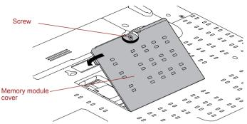
Figure 3-8 Seating the memory module cover
